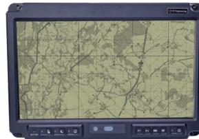
The Rugged Panel Computer (RPC) optimises space efficiency by combining both display & compute capabilities into a single hardware. Built to IP65 rating, the RPC is resilient to environmental factors (e.g., shock, dust, water, temperature), allowing it to perform robustly even under tough conditions.
